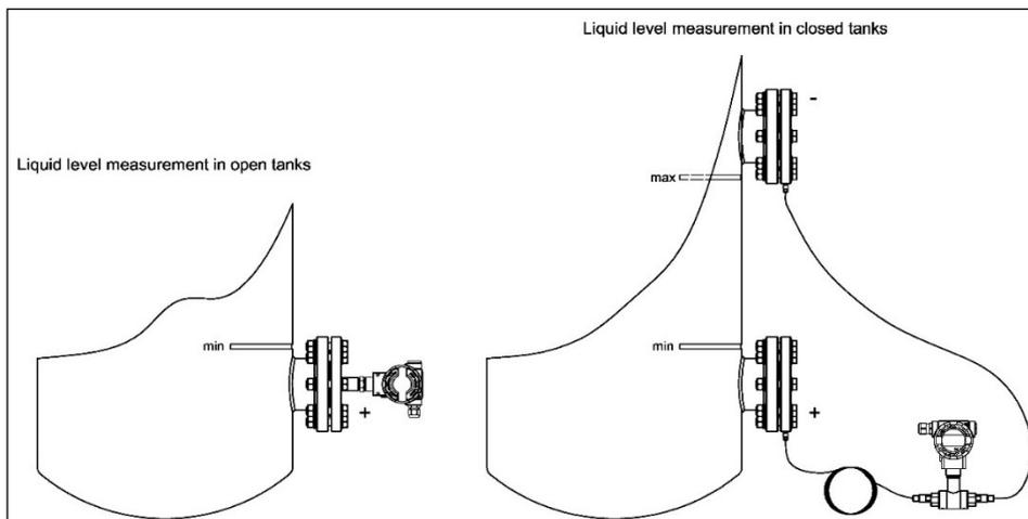
Figure 4. Examples of transmitter installation on tanks
