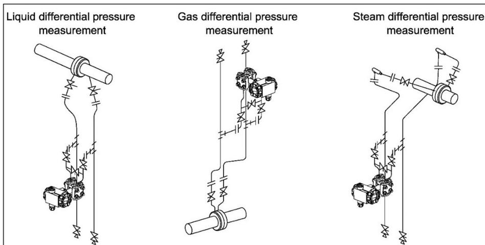
Figure 3. Examples of differential pressure transmitter installation
