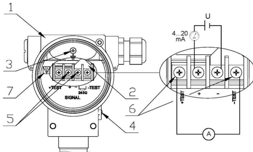
**Figure 5.** Electrical connection to transmitter
