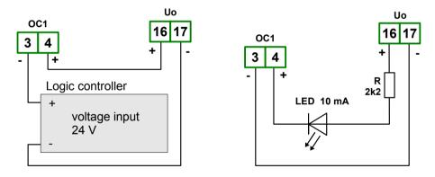
Figure 4.9. Example of OC-type outputs connection
