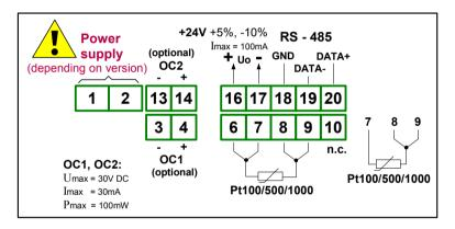
Figure 4.6. Terminals description (OC-type outputs)
