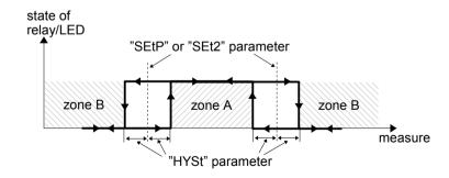
Figure 6.3. Two threshold control of the relay/LED outputs
