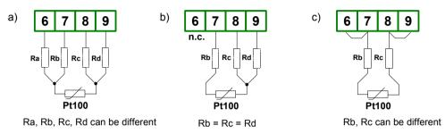
Figure 7. Connection of sensors:
