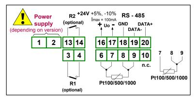
Figure 4.5. Terminals description (relay outputs)
