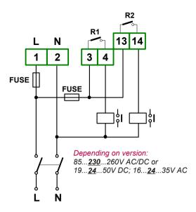
Figure 4.7. Connection of power supply and relays
