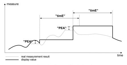
Figure 6.1. Process of peaks detection
