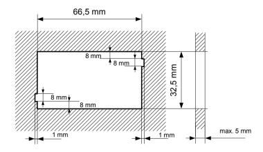
Figure 4.1. Mounting hole dimensions
